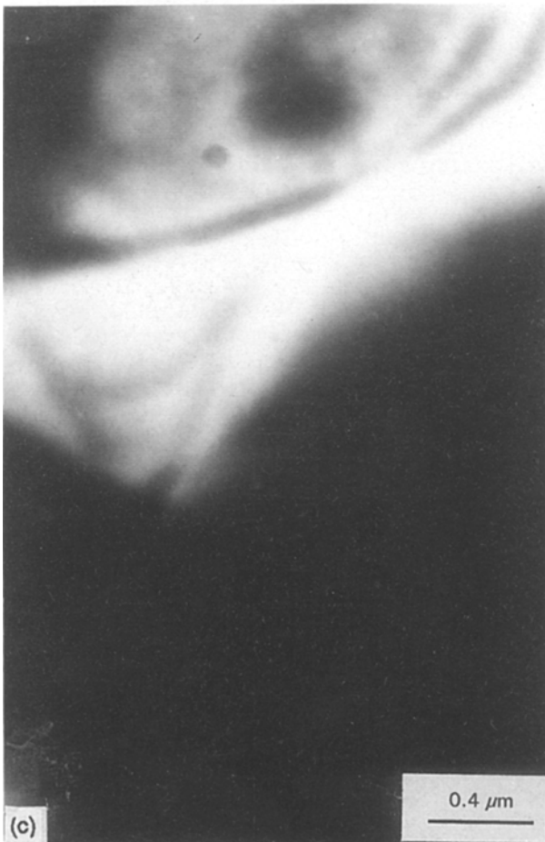
Figure 7 TEM photographs of samples containing 20 vol% Ag: (a) area containing Ag, (b) impurity grain boundary, (c) clear grain boundary. EDX analyses: (d) in area containing Ag, (e) in impurity grain boundary, (f) in clear grain boundary, (g) within one \text{YBa}_2\text{Cu}_3\text{O}_{7-\delta} phase grain.
